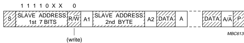
Fig.26 A master-transmitter addresses a slave-receiver with a 10-bit address.
